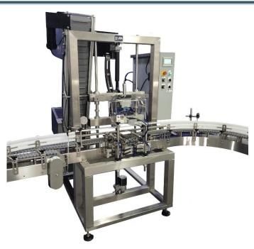
Bartop Corkers use a corking head to press down corks, T-corks and similar closures as bottles pass through the capping area. Automatic corkers use a cork delivery system to seal bottles as they pass on a power conveyor. Bottle corkers are seen mostly in the distilled spirits, wine and olive oil industries but can be used for any product sealed with a cork-like closure.
